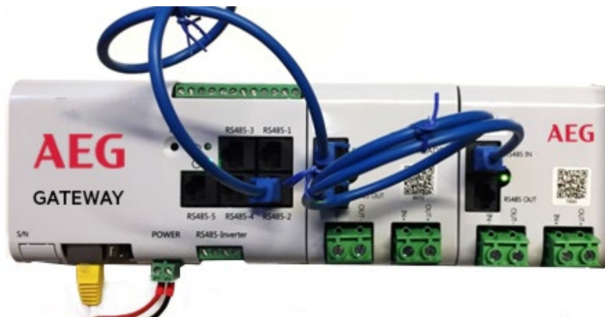
Figure 7: Multidrop connection of String Readers using RJ45 connectors
