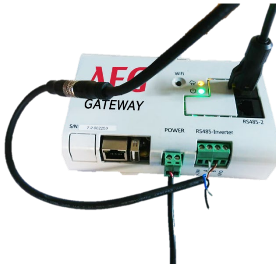
Figure 16: Port configuration for testing
